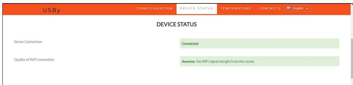
If the quality of the WiFi connection is not optimal, it is advisable to bring USBy close to the Modem / Router and check the status again after a minute of waiting.
